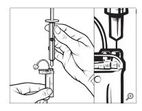
4. Keeping the syringe vertically aligned with the cartridge, and the needle inside the fill port, pull back on the plunger until it is fully retracted. This will remove any residual air from the cartridge. Bubbles will rise toward the plunger.
